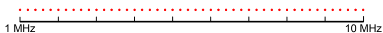
Figure 7-2: Linear x-axis scaling: the distance between the measurement points is equal, e.g. 200 kHz
