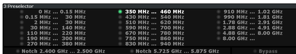
Figure 7-1: Preselector result display. The green LED indicates the currently applied filter.
